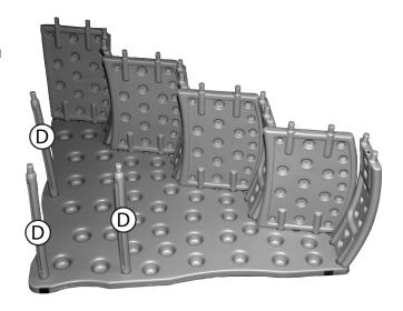
Step 10 Attach left panel, part (A). Align all holes before pushing panel down. Make sure there are no gaps between parts after inserting.
